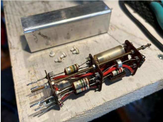
Above top left/right: disassembled 'AGC Assembly' – note the small signal selenium diodes
