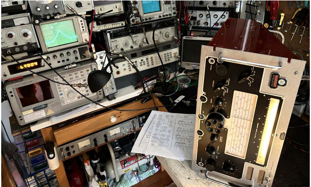
Above: checking the shape of the 85KHz IF response curves using an HP8601A/HP8600A sweeper/markers generator, displayed on a Tektronix 604 monitor (upper left quadrant of this photo)
