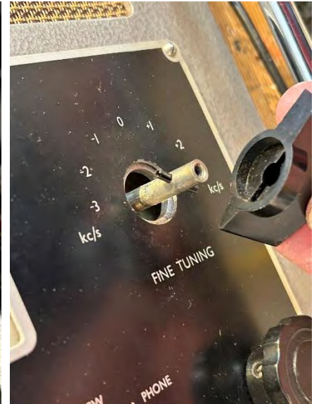
Above left: the cover for the RF deck provides a lot of useful location information. Above: all of the knobs, except the AF and RF gain controls, are screwed and keyed onto their shafts. Below left: view inside the cabinet after wiring-in the 110vDC line and filter ground wire. Below: the static discharge resistor across the antenna socket
