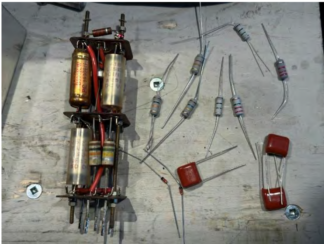
Above: assembling the parts needed to replace the components in the 'AGC Assembly' (I subsequently decided to use axial lead capacitors as these suited the layout better)
