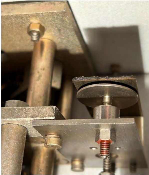
Above: the rear of the tuning gang cover looks like it should be attached to the end plate of the tuning gang – but its not(!). Left: the adjustable air-spaced temperature compensation capacitor across the 1 st local oscillator section of the tuning gang. Below: the (above chassis) RF deck trimmers and slug adjuster screws – a 'twiddlers delight'...
